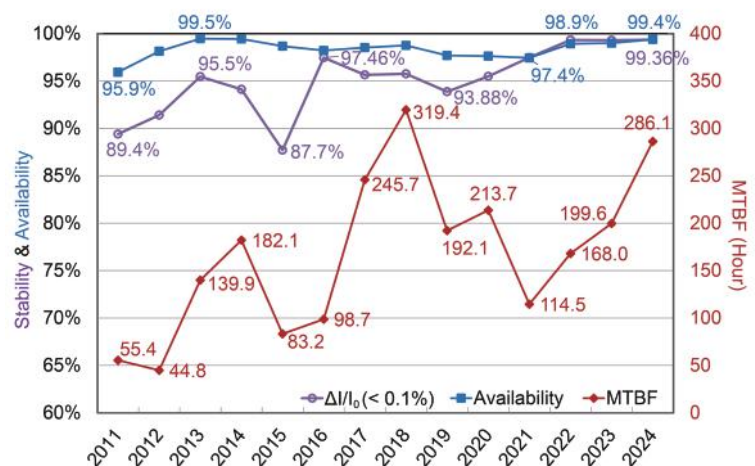
Fig. 1: Annual beam stability index of 0.1%, availability, and MTBF of the TLS.
