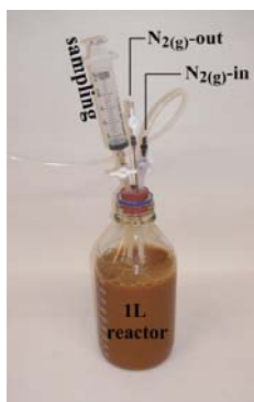
Fig. 1: Photograph showing the set-up of the anoxic transformation experiments used to evaluate arsenic effects and behaviour during the \text{Fe}^{2+} -catalysed transformation of schwertmannite to goethite. All experimental runs involved 5 g of schwertmannite suspended in 1 L of 0.1 M NaCl, buffered at pH 6.5.
