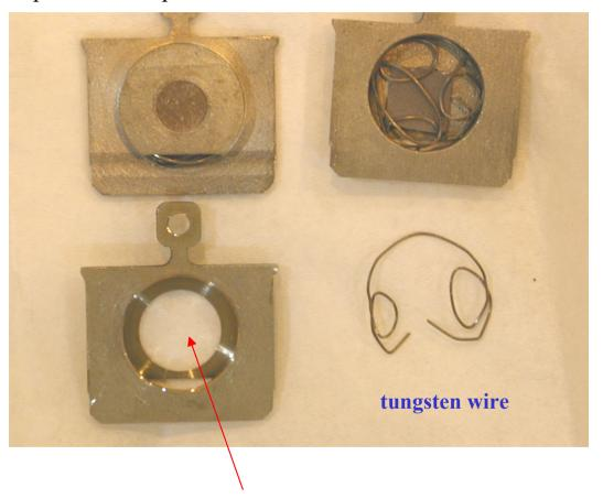
Sample plate with different center opening (5mm, 6mm, and 8mm) are available.
