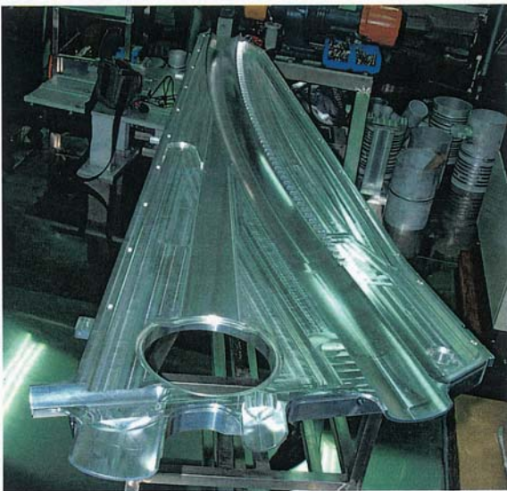
Fig. 3: A half piece of the B-ch after oil-free CNC machining.
