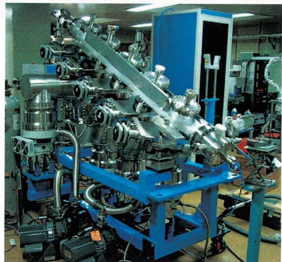
Fig. 6: Photograph of the gas filter system for 03(HF).
