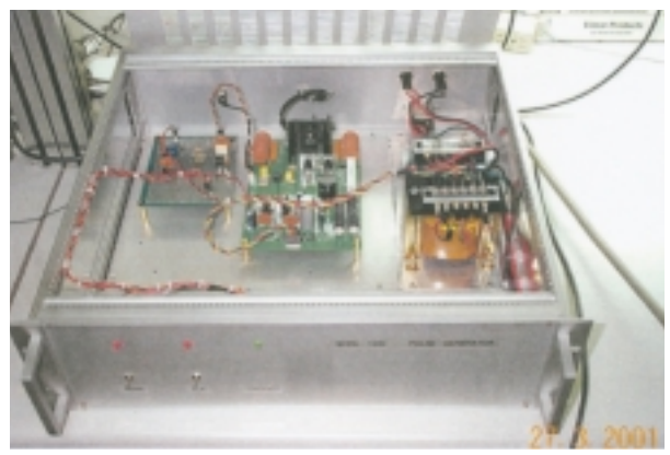
Fig. 7: Inside the SRRC-1000 thyatron pulse driver.
