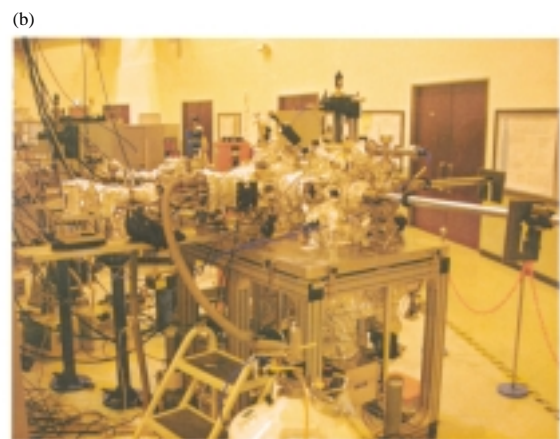
Fig. 2: (a) Schematic drawing of PEEM station. (b) Photo of PEEM station at the EPU-SGM beamline.
