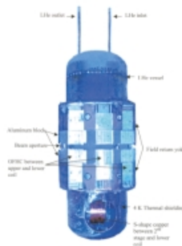
Fig. 1: Components of the 4 K cold mass inside the cryostat of the superconducting wavelength shifter.
