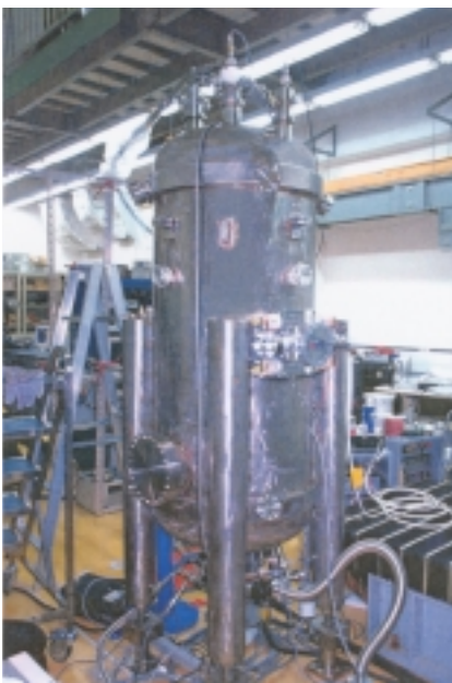
Fig. 2: Photograph of the SWLS magnet and the Hall probe magnetic field measurement system.
